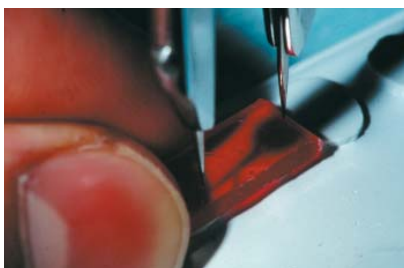
5. The scratching of r_1 and r_2 with dividers for the planned rotation of the lock blade and the lock nose.
