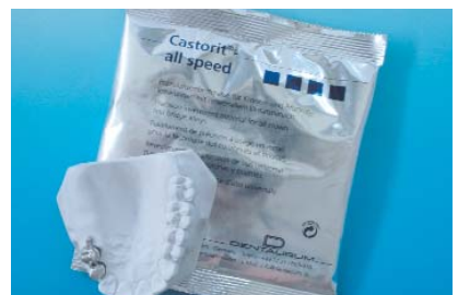
19. The cast crowns have been invested with Castorit all speed. That's an investment material for C&B technique with a maximum expansion of 3.3% for casting CoCr alloys or precious alloys.
