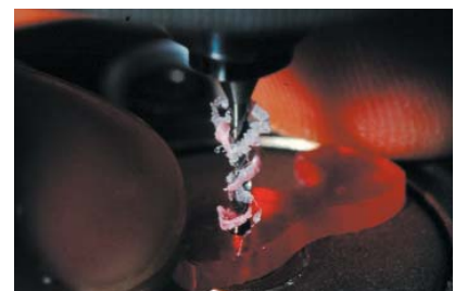
7. The drilling of the axis hole (diameter 1.5mm).
