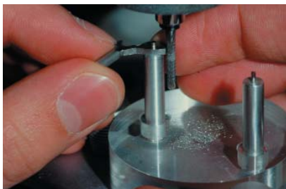
14. The milling of the CoCr lock. The lock is turned in a clockwise direction against the cutters of the milling tool with a fixed milling arm of the milling machine. The lock blade is finished after the milling of the stopper.
