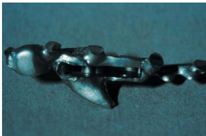
23. The view into the lock housing after casting with remanium star.
