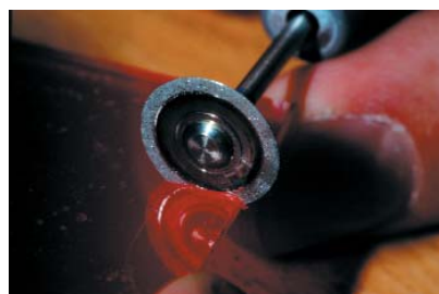
3. Cutting of an acrylic blade according to the lock size.
