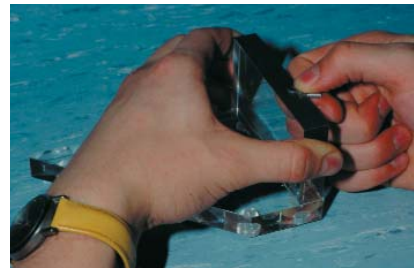
13. The handling of the lock-smoothing tool. The surface of the lock is smoothed with strips of different abrasive papers (corn sizes 240, 500 and 1200).
