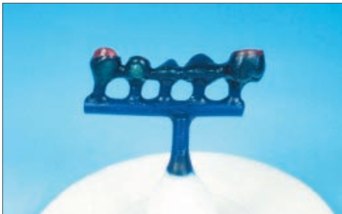
Fig. 1a,b: Spruing systems for titanium castings (Rematitan)
