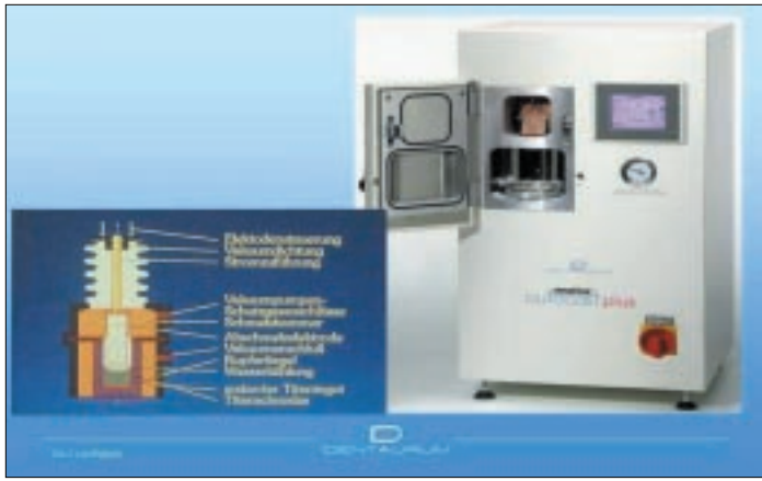
Fig.2: industrial and dental casting equipment (Dentaurum) for titanium
