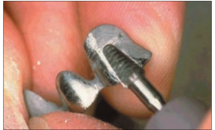
Fig.4a,b: Tungsten carbide cutters, cross shaped cutting edge (Dentaurum)
