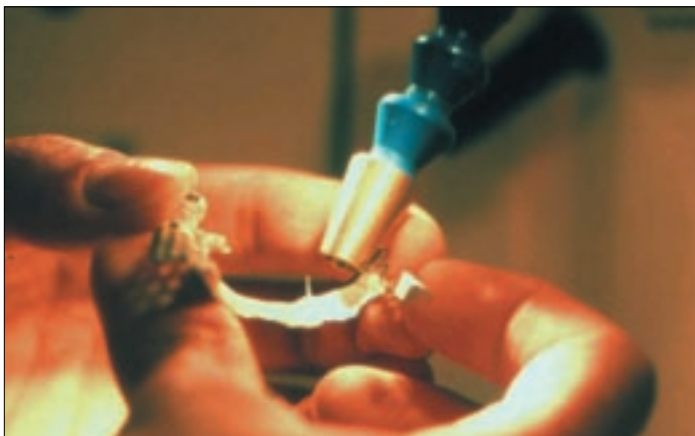
Fig.5a,b: Adjustment of argon gas, avoiding discoloration of laser spot
