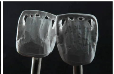
Fig. 3 - Holes made manually with fisher burr at the green stage to define the translucent spots like the ones on the natural adjacent teeth
