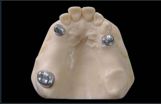
Figure 3. Primary crowns cast with remanium star after milling.
