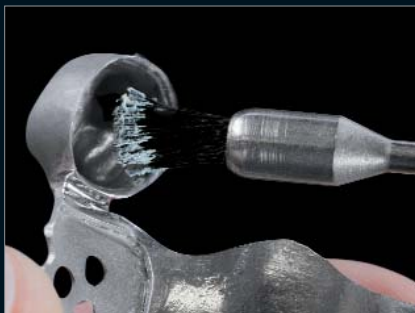
Figure 28. Fine-fitting the secondary crowns with a pointed brush and Tiger brilliant polishing paste.
