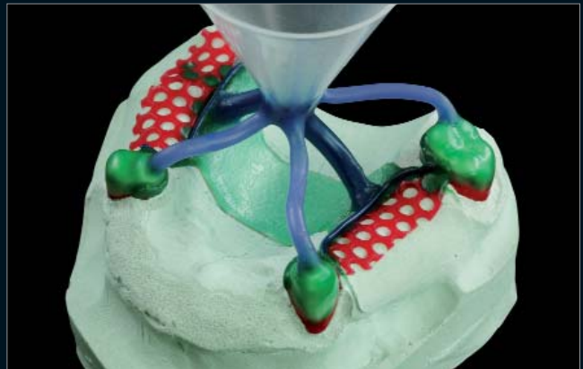
Figure 21. Main sprues with diameter 3.5mm.
