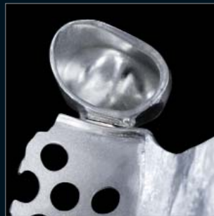
Figure 26. Processed crown margin.
