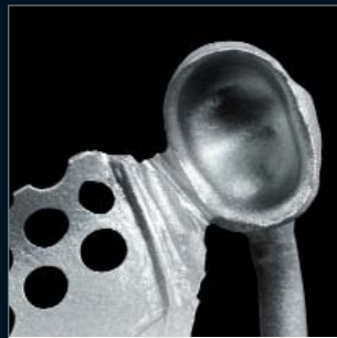
Figure 25. Crown margin after casting.
