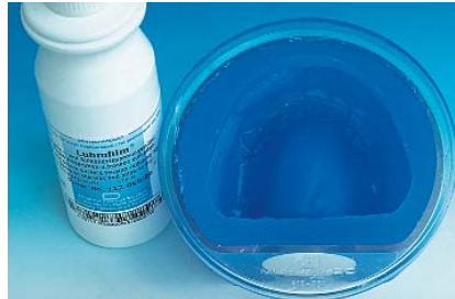
Figure 9. Silicone duplication with rema®Sil and surface tension reducing agent Lubrofilm.
