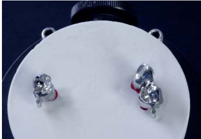
Figure 5. Primary crowns after casting with remanium® star on the milling base.
