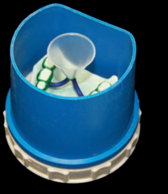
Fig. 6: Sprueing the wax-ups with 3.5 mm thick sprues.
