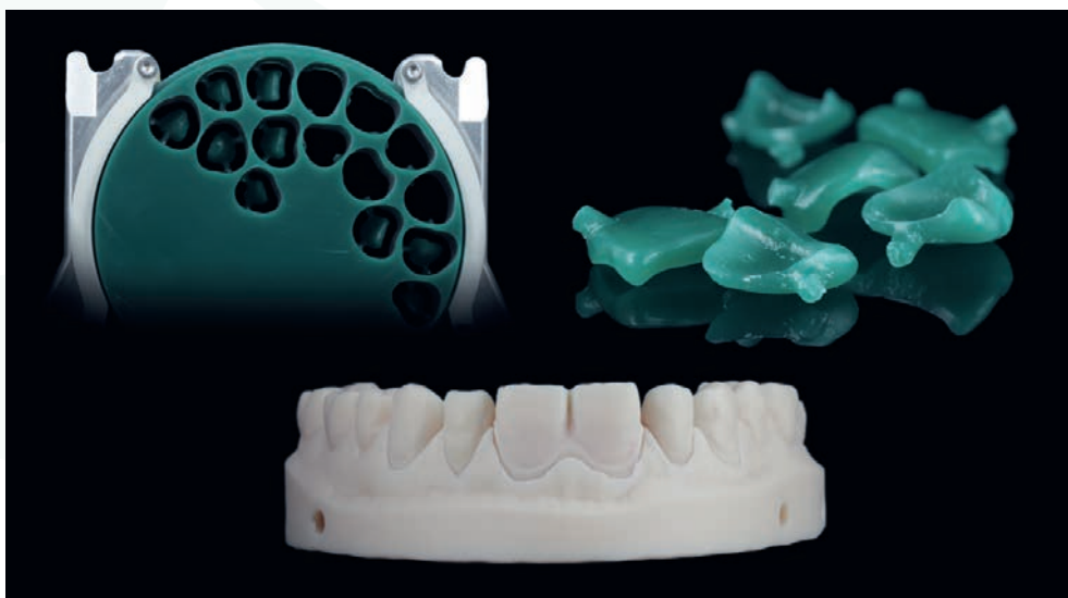
Fig. 6 — The modified veneers are milled from a burn-out wax using the new construction data.
