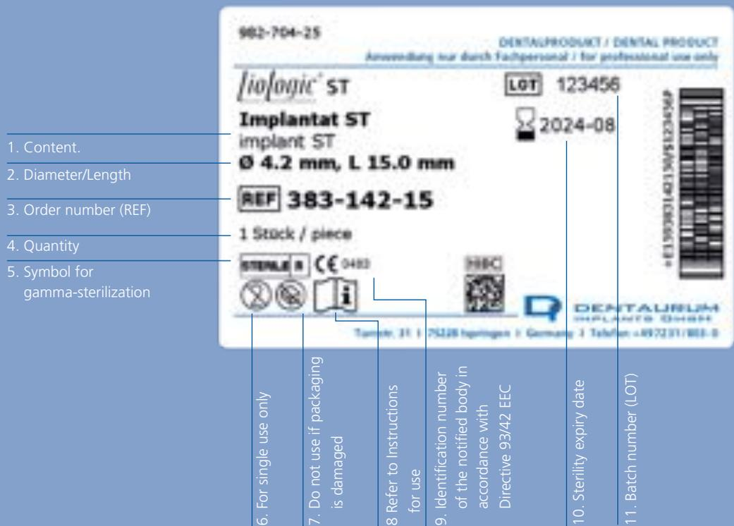
All tioLogic® implant types are supplied individually with a closure screw and in gamma-sterilized double packaging. They are intended for single use only. The double packaging (foil and blister packaging) protects the inner container with the sterile implant and closure screw against contamination. The contents remain sterile as long as the packaging is undamaged. The product should not be used if the double packaging is damaged.
