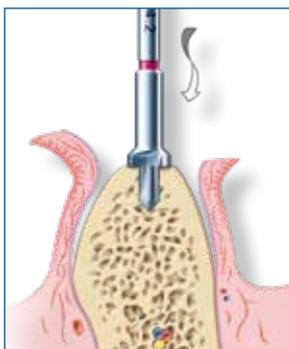
The shape of the **surface cutter STANDARD** has been specially designed for drilling through the compact bone and for preparing a flat bone surface cervically. It has a color-coded groove, which indicates the planned final implant diameter (here red for  $\varnothing$  4.2 mm) and is used for all lengths of implant. The implant diameter is also laser-printed on the surface cutter.
