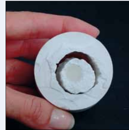
Fig. 24: blasting the inner cylinder of investment
