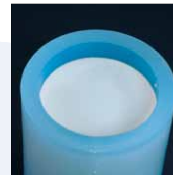
Fig. 13: fill with investment material up to the marked point
