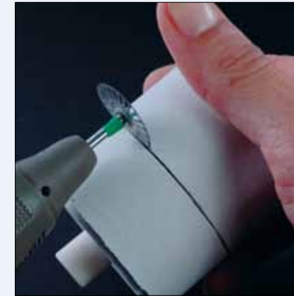
Fig. 21: cutting with a separating disc
