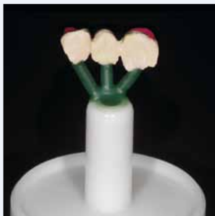
Fig. 12: sprues on the ring base
