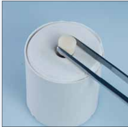
Fig. 18: placing the press pellets into the channel
