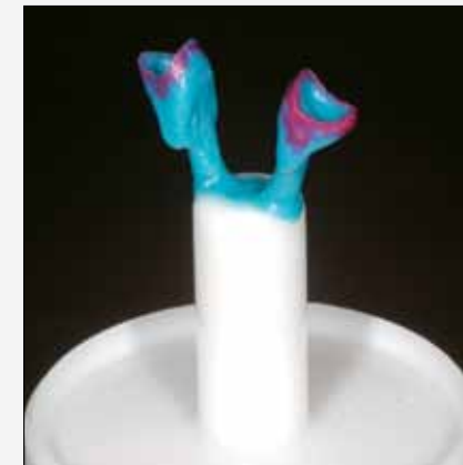
Fig. 5: sprued objects on the ring base
