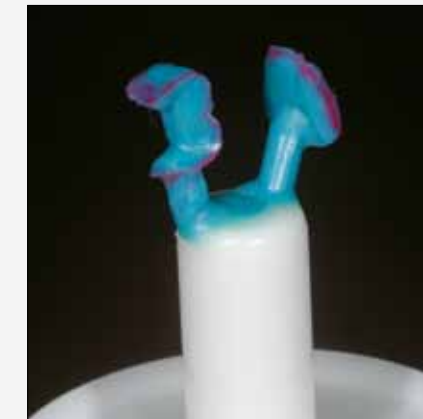
Fig. 6: sprued objects on the ring base
