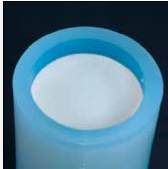
Fig. 7: fill with investment material up to the marked point
