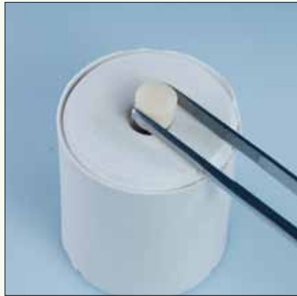
Fig. 16: placing the press pellets into the channel
