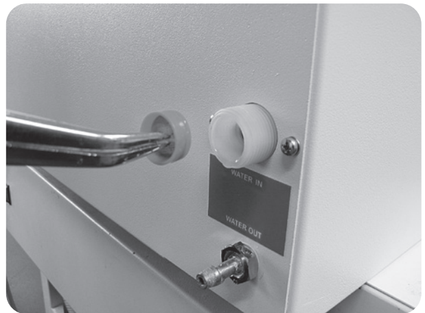
Fig. 5: Installation position of the water filter on the fresh water connection
