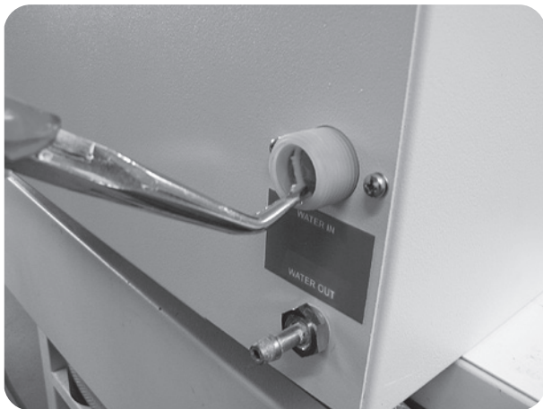
Fig. 5: Installation position of the water filter on the fresh water connection
