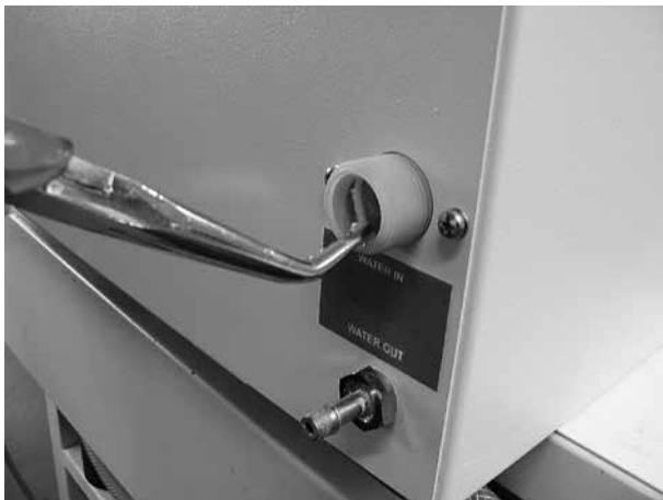
Fig. 5: The water filter is fitted at the fresh water inlet
