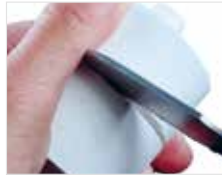
Fig. 7c) Break at the incision using a plaster knife.
