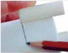
Fig. 7a) After cooling, mark the length of the press plunger on the casting ring.
