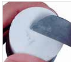
Fig. 6d) Using a plaster knife, smooth out any unevenness.
