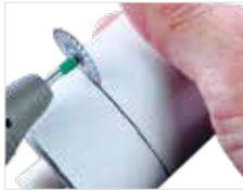
Fig. 7b) Using a separating disc, create a predefined breaking point all around.
