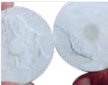
Fig. 7d) Separated casting ring at transition point from plunger to pressing cone.
