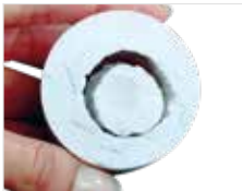
Fig. 7e) Rough devesting with \text{Al}_2\text{O}_3 at max. 4 bar pressure. Careful, precise blasting with glass beads (medium grain size) at max. 2 bar pressure.
