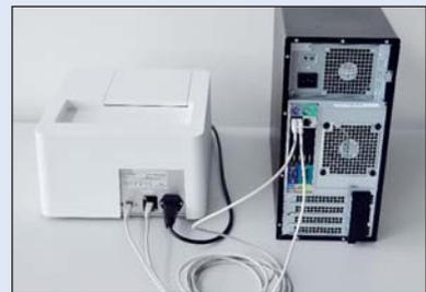
Connect the 3D model scanner with the computer using the USB cables.
