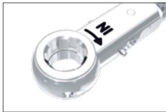
Ratchet head, assembled.
