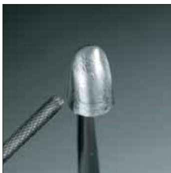
Fig. 1: Metal surface ground with a cross-cut tungsten carbide bur before sandblasting.
