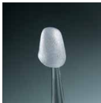
Fig. 2: Surface sandblasted with 110 – 150 µm at 2 – 3 bar pressure.
