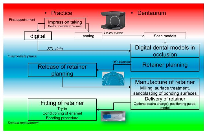
Fig. 6 Overview of the sequence of the individual process steps for using CAD/CAM manufactured retainers
