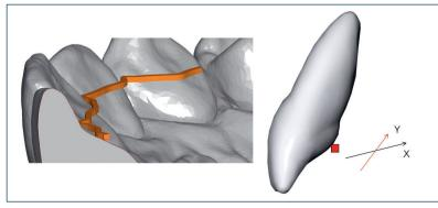
**Fig. 4** An arch made from square wire that cannot be changed vertically can never lie fully on one or more inclined planes (palatal surfaces of the teeth). It can only be in contact with a corner of the profile of the inclined plane's surface. There is therefore always an empty space in a triangular form that depends on the angle between the square wire and the tooth surface.
