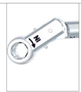
The pressure point for exact torque release is at the head of the torque adjustment screw. When the set torque has been reached, the scale sleeve will bend around the ratchet head axis. The release is audible and perceptible. After the torque release, **DO NOT** apply more pressure as this could damage the ratchet.
